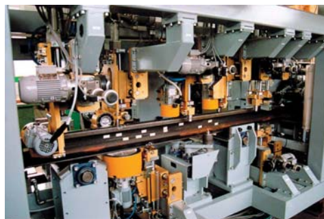
Eddy-current system for testing rails for surface flaws with rotating disks CIRCOGRAPH® and shape-adapted segment coils
